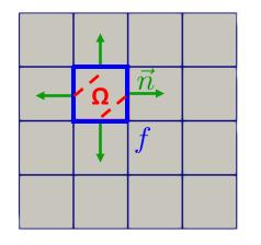
FVM = integration of the flow equations over a control (finite) volume (Ω)
