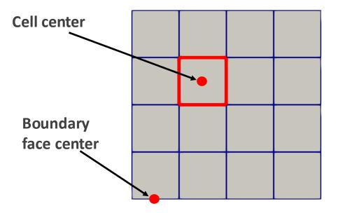
Flow quantities are computed/stored at the cell centers and boundary conditions are imposed on the boundary face centers
